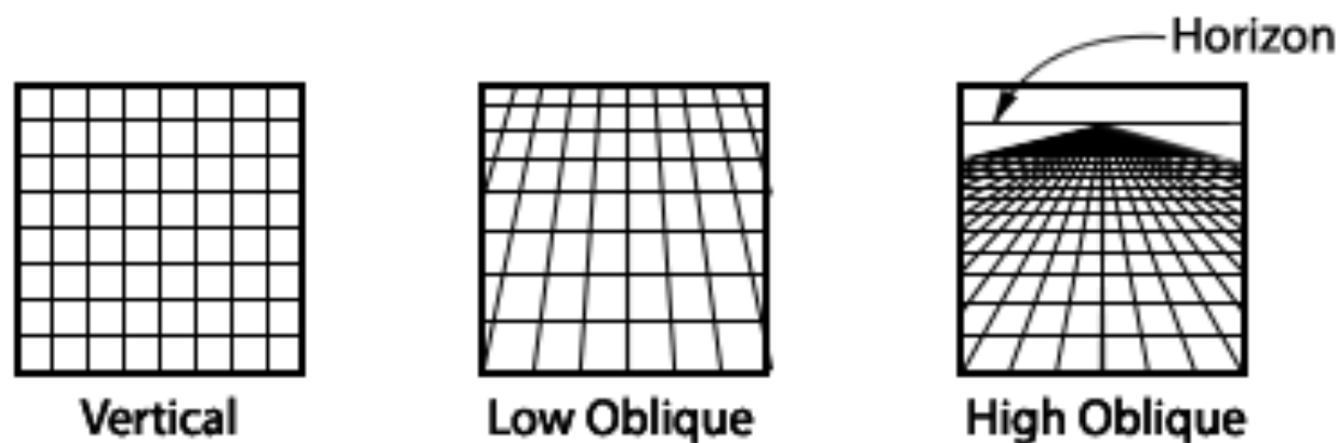
How a grid of section lines appears on various types of photos.
